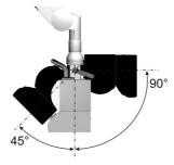
Every IR-modules has a clamping joint that approve 90° and 45° overturning as shown above. Using IR-modules with additional ball joint you get countless positioning options.
