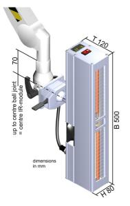
IR-module type 2x 0.8 kW; 230V (50/60 Hz)**Extremely small design**, therefore suitable for drying work at difficult to access<br/>parts, for example in the vehicle door area.With additional ball joint for positioning in all directions.Drying surface approx. 450x200mm (width x height) at a working distance of 55cm<br/>Colour:Colour:alu nature anodised<br/>6.0 kgitem-no.:600.2210.4
