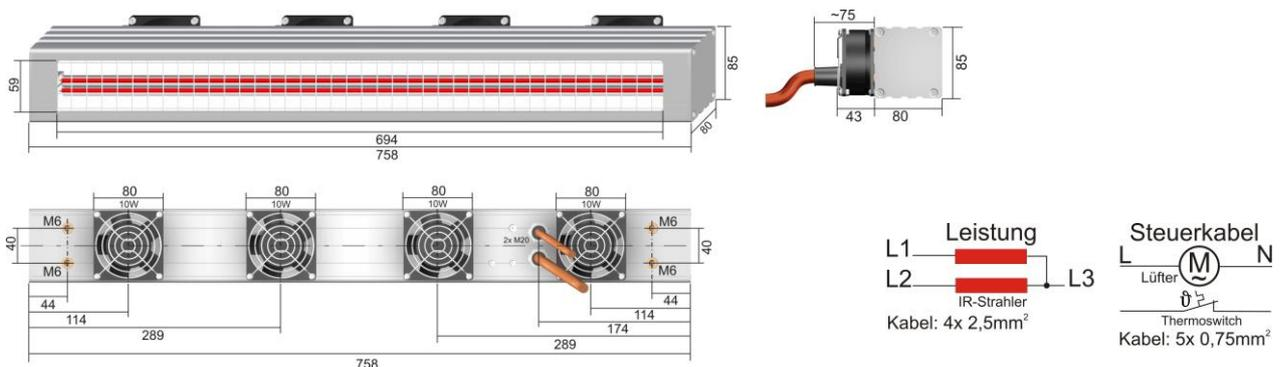
**IRD E750Z** – 2x 3 kW / 400 V + N + PE (50/60Hz);
