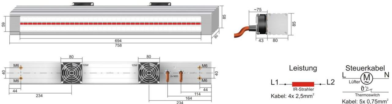
**IRD S750** – 4 kW / 400 V + N + PE (50/60 Hz);
