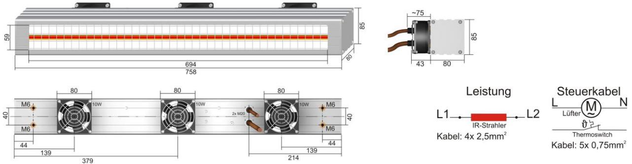
**IRD S750Z** – 2x 3 kW / 400 V + N + PE (50/60 Hz);
