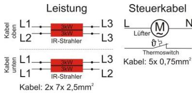
**IRD E1121Z** – 2x 6 kW / 400 V + N + PE (50/60Hz);
