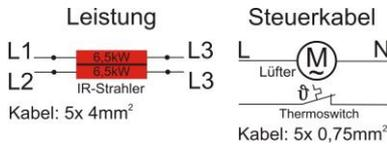
**IRD E2140Z** – 2x 13 kW / 400 V + N + PE (50/60Hz);
