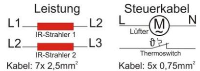
**IRD E750D** – 3x 3 kW / 400 V + N + PE (50/60 Hz);
