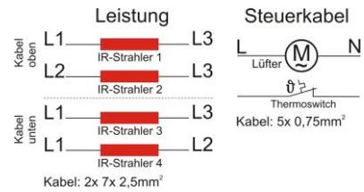
**IRD S1121** – 6 kW / 400 V + N + PE (50/60Hz);
