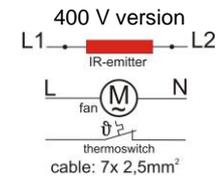
**IRD E540Z** – 2x 3 kW / 400 V + N + PE (50/60Hz);
