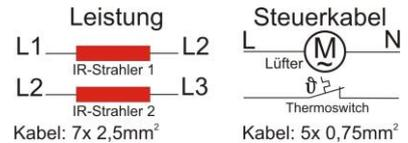
**IRD E750Z** – 2x 3 kW / 400 V + N + PE (50/60Hz);
